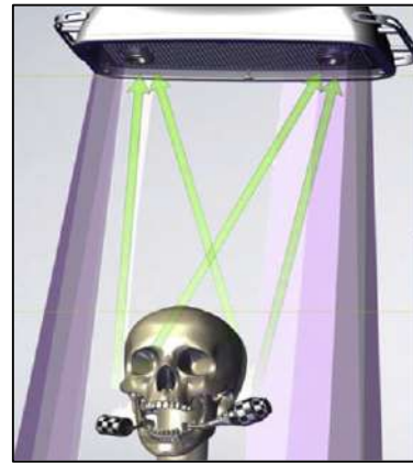
Figure: 1 : The patient and drill must be over the line of sight of the tracking camera
